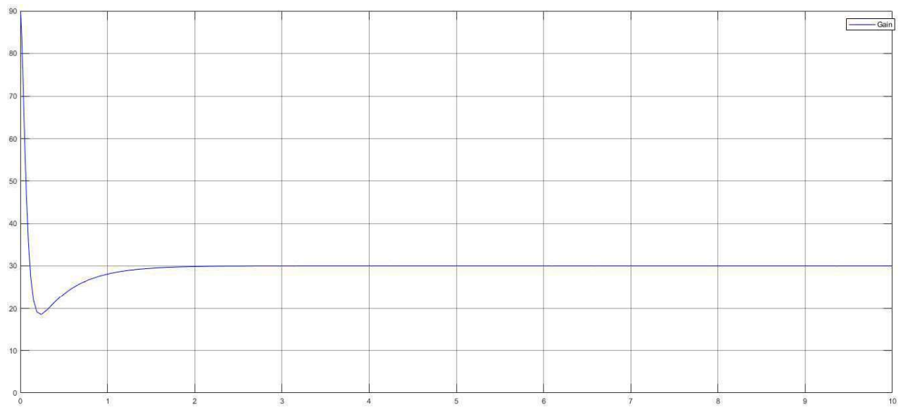
Figure 7: Angle of the single link manipulator over time
